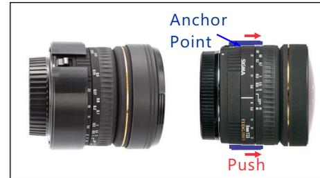
Align the slit on the inner ring to **AF/MF** switch on lens. Insert the lens. Stretch the ring when necessary. Move it to a position where it fits snugly. Keep even spacing between the slit and **AF/MF** switch. Push it against the anchor point to ensure reproducible mounting and consistent NPP settings.
