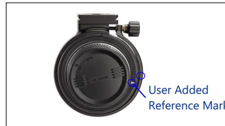
Align the outer ring to the slit of inner ring. Insert the outer ring (loosen its knob further if needed) from the back of the lens. Tighten its knob slightly. Rotate the outer ring so that it snaps to the inner ring and rotates smoothly. Optionally align the notch indicated to the user added reference mark. Tighten the knob fully.
