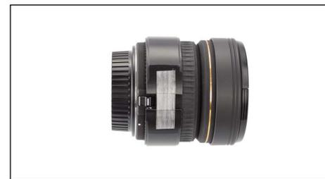
Fix the inner ring with a piece of tape about 40mm (1.5") long. Stretch the tape so that the ring will grasp the lens firmly. This prevents movement of inner ring when outer ring is rotated, thus protecting the paint of lens barrel. Cut any tape that goes beyond the trimmed area of the inner ring.
