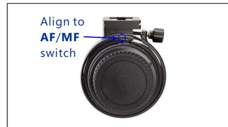
Align the outer ring to the slit of inner ring. Insert the outer ring (loosen its knob further if needed) from the back of the lens. Tighten its knob slightly. Rotate the outer ring so that it snaps to the inner ring and rotates smoothly. Align the notch below the lens ring plate to the **AF/MF** switch. Tighten the knob fully.
