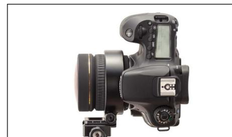
Mount the lens to the camera and it is now ready for use on any Arca Swiss compatible gear. The camera will be in portrait mode with handgrip pointing up. Loosen the knob on the ring to rotate to other angle. Use the notches (at 30° interval) at the back of ring to have accurate roll angle alignment. Use the center of **AF/MF** switch as the reference.
