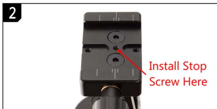
Install the stop screw (came with the stop plate) at the middle socket on the QR clamp. Remove any other safety screw installed. Mount the lens ring on the clamp. Slide until it falls into the stop. Confirm the reading with the published NPP settings.
