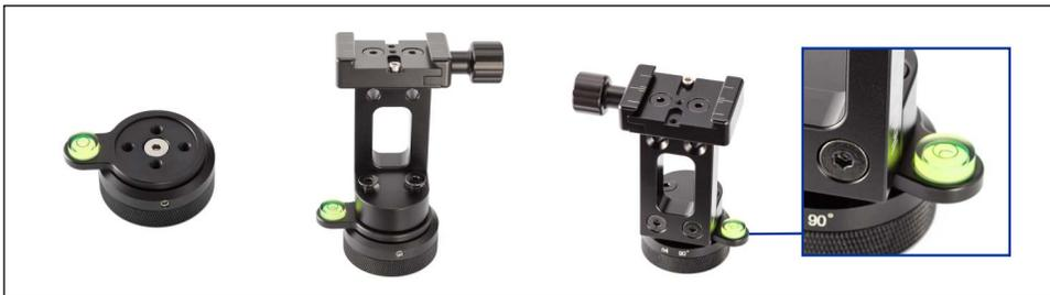
Place the level on RM with bubble facing up. Place R10 tilt head on the level. Align for the mounting sockets. Install 2 M5 flat head screws to fix R10 head to RM. While the level is still movable, turn it to the rear right of R10 for best clearance of view and least footprint. Keep it at 2-3mm (1/8") clearance from R10 to prevent damage of bubble by accidental bumping of bubble into R10.
