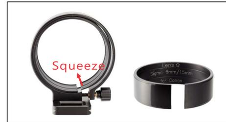
Loosen the knob on the outer ring until its slit is about 6mm (1/4") wide. Squeeze to take out the inner ring. Check the label on the inner ring to confirm with the lens in use and the direction of mounting. The arrow should point to the front of lens.
