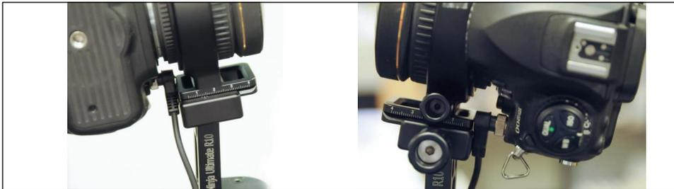
It is reported that lens ring for Sigma 8mm for Nikon blocks the remote port for Nikon D200/300/700 etc.
